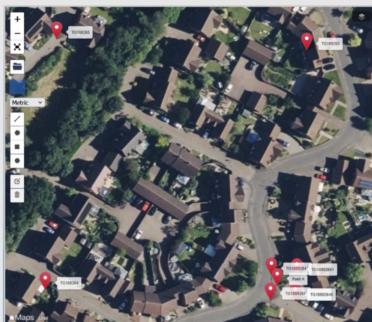
Fig. 4. Here's what happens when you step up to an eight-figure grid reference. Retaining the same screenshot to show the 100x100m square, I've now added in the 10x10m square that we get by using eight figures for our grid reference. Point A is still present in the bottom right corner and we can also see the tight cluster of markers around it.
