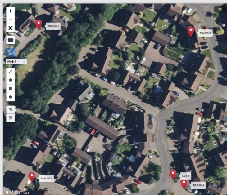
Fig 3. In this screenshot, I have left the marker for Point A in place (now in the bottom right corner of the picture). I have also now added the marker for the six-figure grid reference TG188264. The mapping system will place this point at the bottom left corner of the area covered by that six-figure reference. That is, at the bottom left of a 100x100m square. By advancing the reference by one digit north and east and dropping more markers, we can demonstrate the entire 100x100m square. Thus, by sending someone this six-figure reference, we are saying 'The plant is somewhere in that area'... that's a lot of pavement edge to search!
