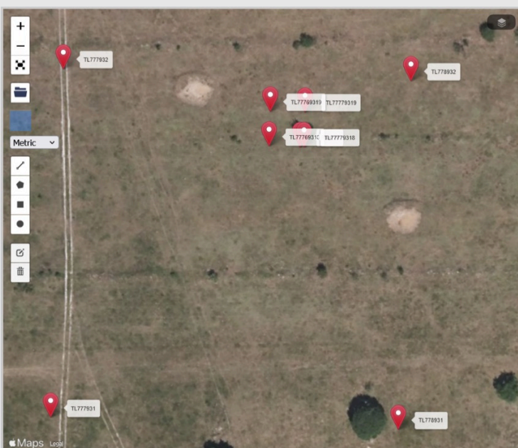
Fig. 9. Here the eight-figure grid reference is used to show the 10x10m square within the six-figure, 100x100m square. Again, quite a difference when it comes to a search area.
